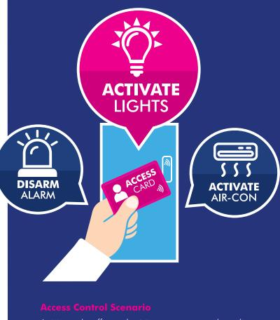
Arriving at the office and swiping your access card can disarm alarm, activate lighting & air conditioning.
